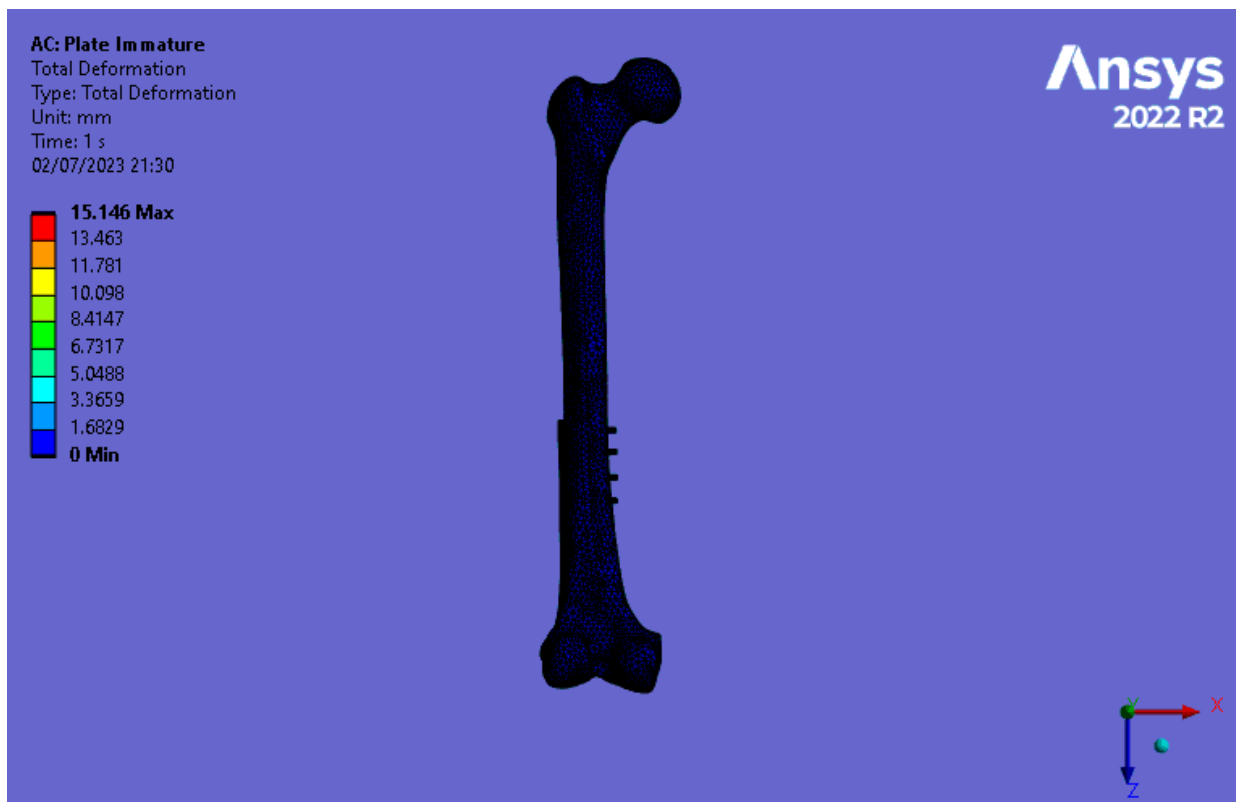
Figure 4.6 Plate Immature - Full Load – Deformation
