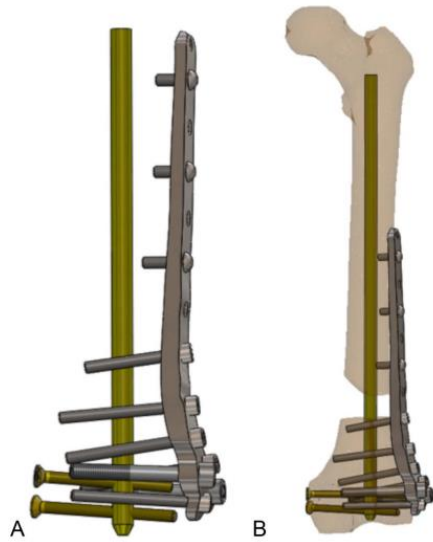
Figure 2.12 Combination of Nailing System and Locking Plate [12]
