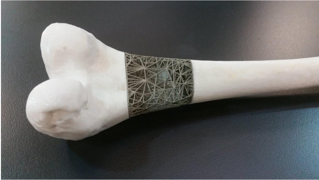
Figure 2.16 Metallic 3D Printed Implant on Distal Femur
