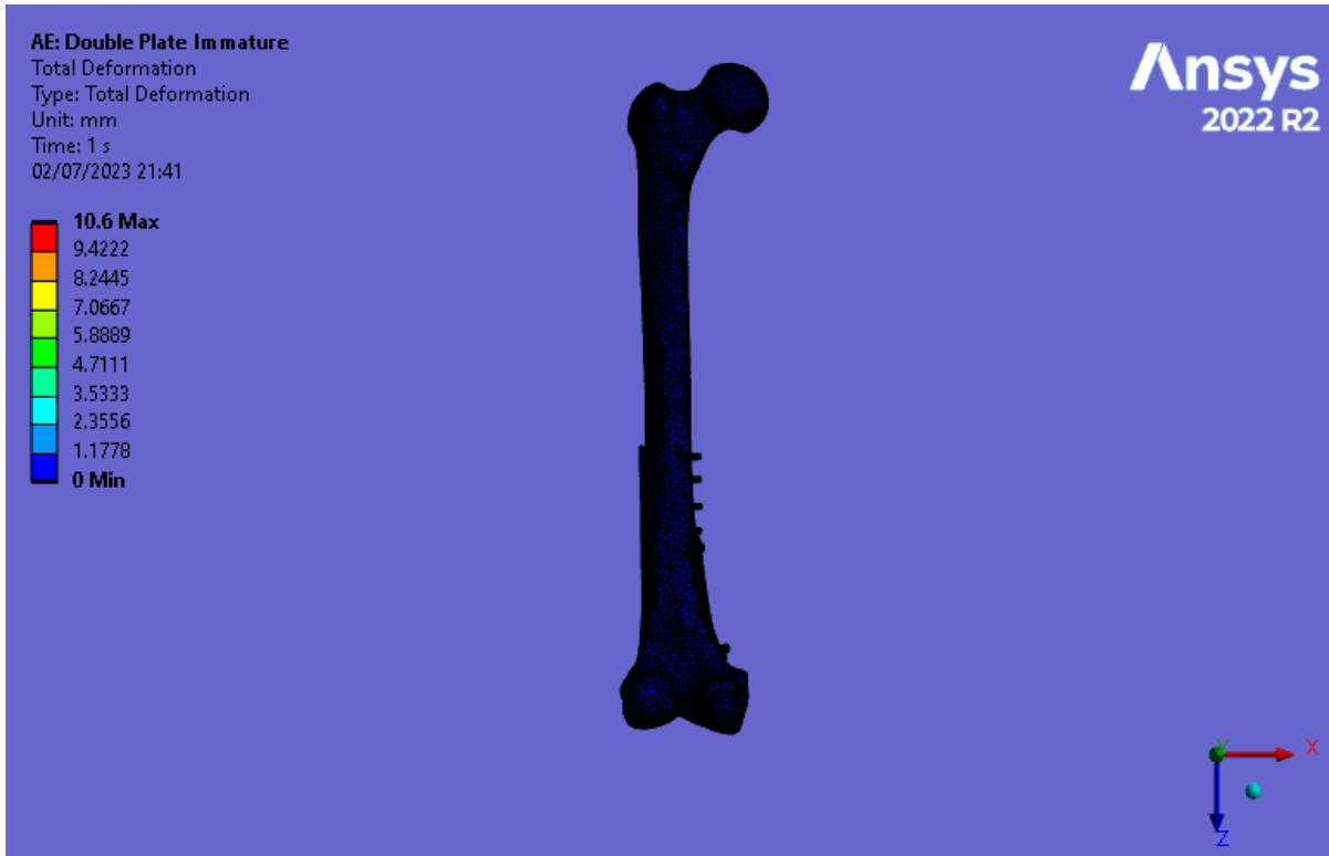
Figure 4.7 Double Plate Immature - Full Load – Deformation
