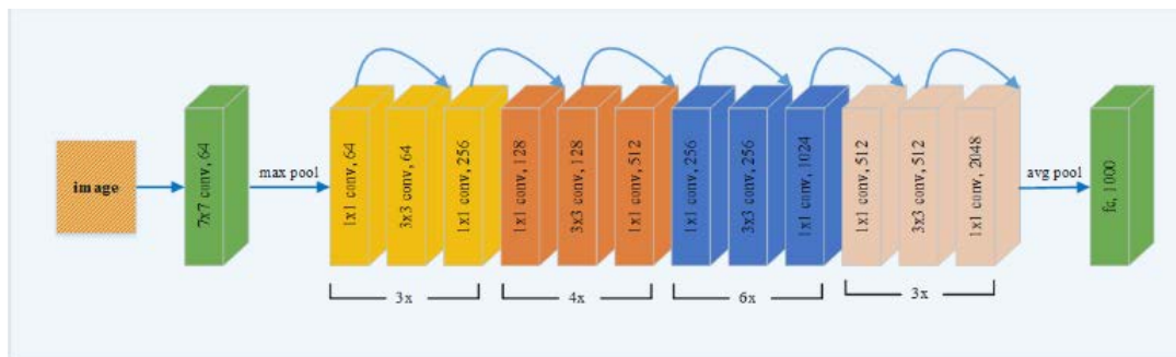
Figure 13. A block diagram representation of pre-trained Resnet-50 architecture.
