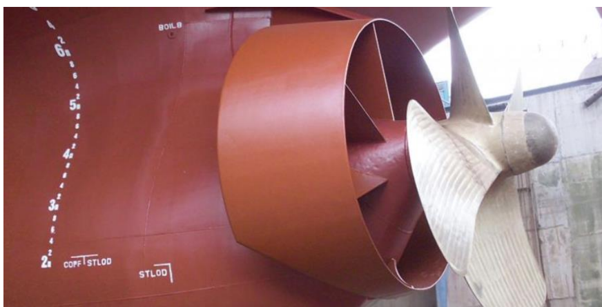
Figure 24: Pre-swirl duct fitted in front of a propeller. [57]
