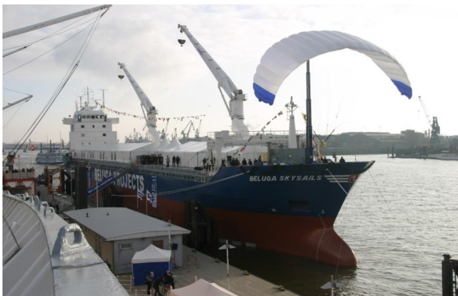
Figure 16: Applied computer-controlled kite rig on a Multi-Purpose General Cargo Vessel.
