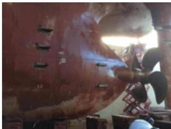
Figure 27: Vortex generators installed on the vessel's hull. [60]
