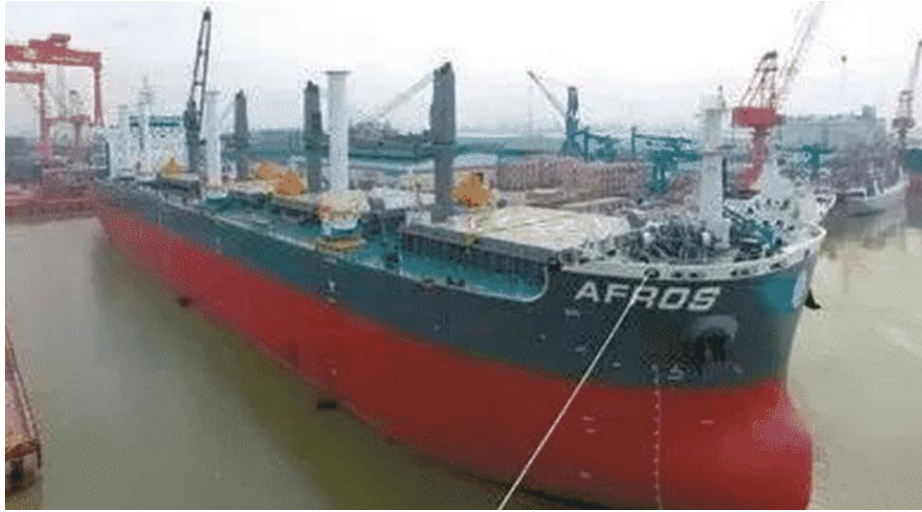
Figure 15: Rotor sails fitted with rotor sails.
