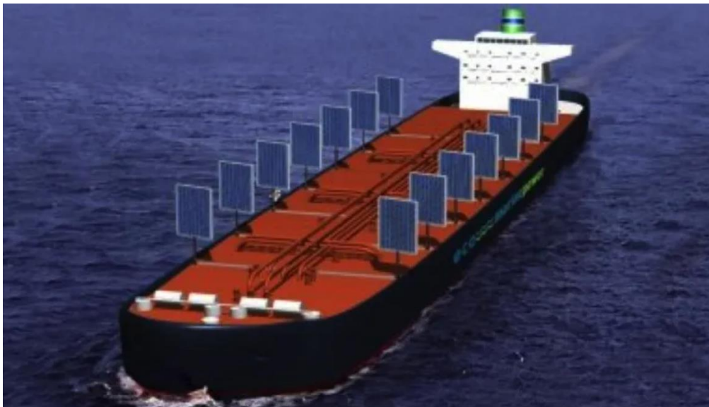
Figure 17: Solar panels on a tanker.
