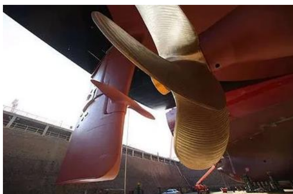
Figure 29: Thrust fins fitted on a rudder.
