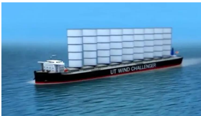
Figure 14: Bulk Carrier equipped with wing sails.
