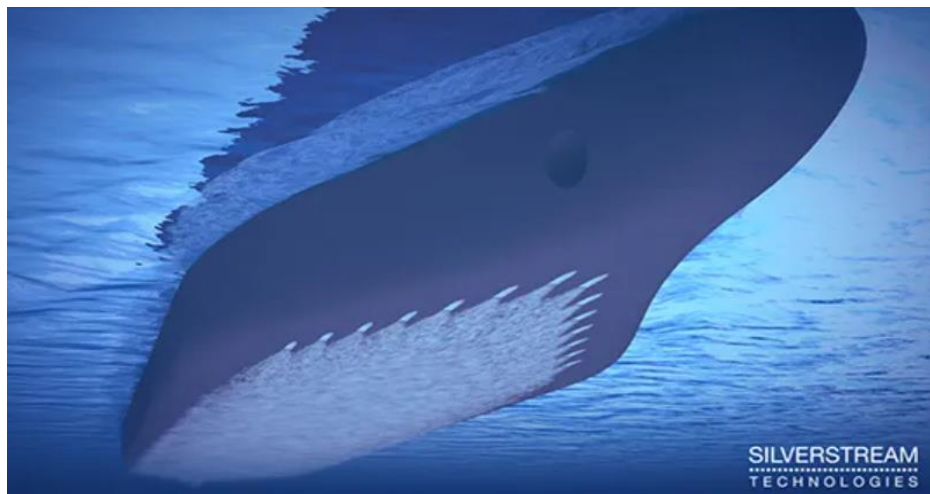
Figure 18: Carpet of microbubbles produced by an Air Lubrication System. [51]
