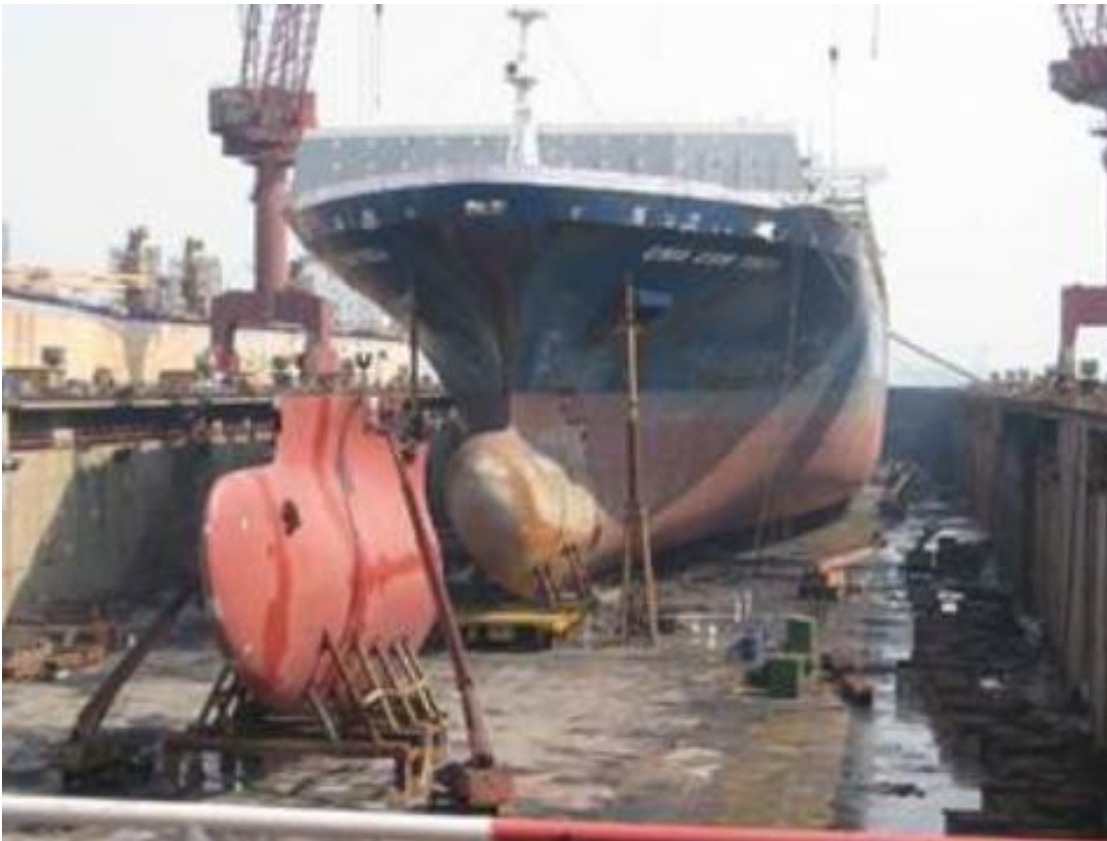
Figure 21: Retrofitting of bulbous bow for a container ship.
