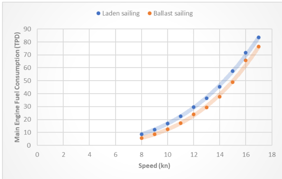
Figure 63: Fuel oil consumption at tons per day versus speed graph of the VLOC when in laden and ballast mode.
