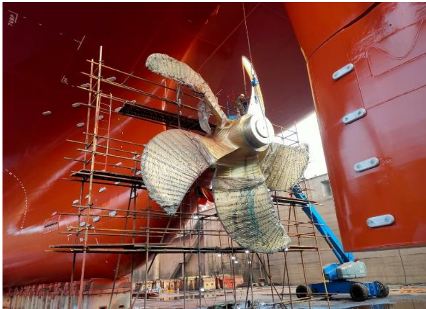
Figure 22: Propeller retrofitting during drydock. [55]
