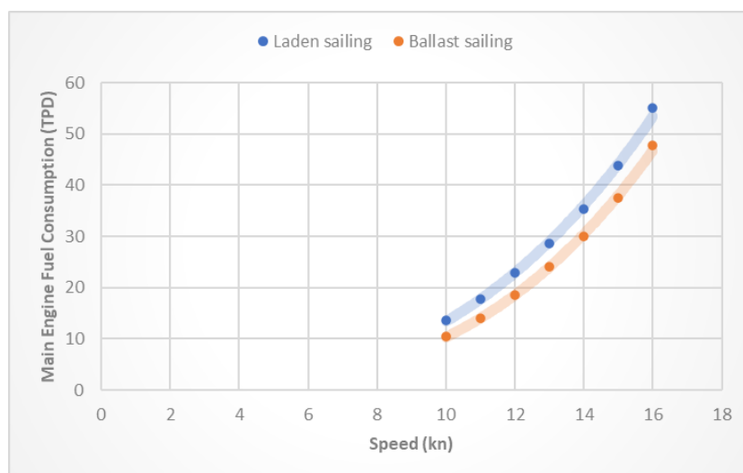
Figure 42: Fuel oil consumption at tons per day versus speed graph of the Aframax tanker when in laden and ballast mode.
