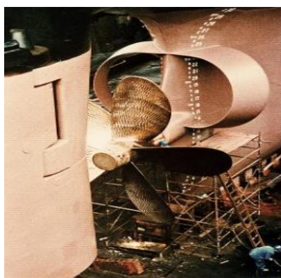
Figure 30: Wake Equalizing Duct fitted forward of the propeller.
