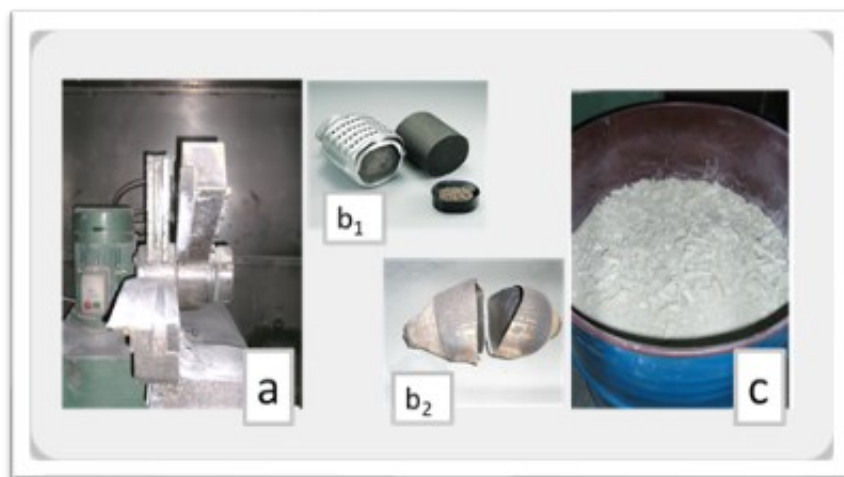
Figure 2.4: (a) Automatic cutting machine for the ceramic catalyst decanning, removal of metallic case preserving the shape of the cordierite (b2) empty case of ceramic catalyst and (c) crashed ceramic honeycomb.
