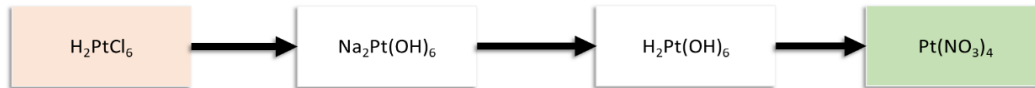
Figure 4.5: Flowsheet of the steps followed for the conversion of Pt chloride species into nitrates.
