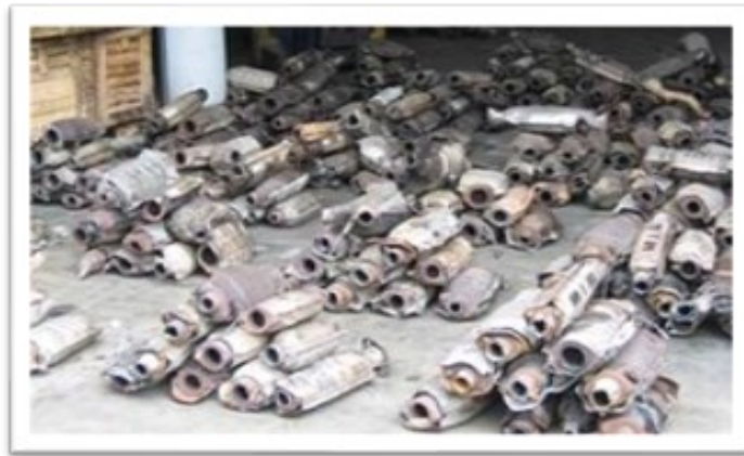
Figure 2.3: Sorting of the collected spent/deactivated catalyst according to certain criteria
