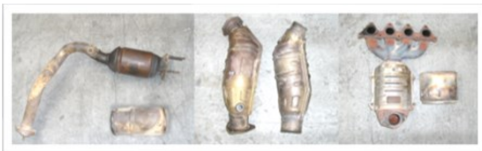
Figure 2.2: Inlet and outlet exhaust tubes are removed from the main body of the catalyts during the shredding procedure
