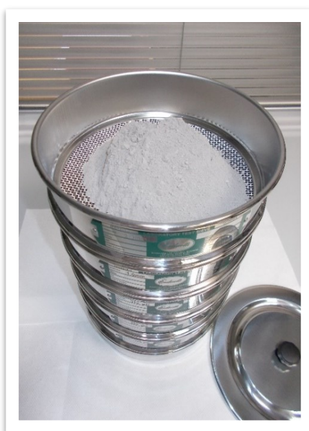
Figure 2.7: Sieving of the obtained sample to determine granulometry
