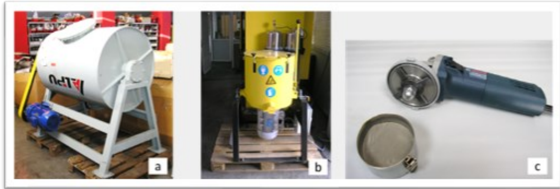
Figure 2.5: (a) Ball mill, (b) chain mill and (c) analytical mill used for the downsizing of the ceramic monolith particles before the analysis
