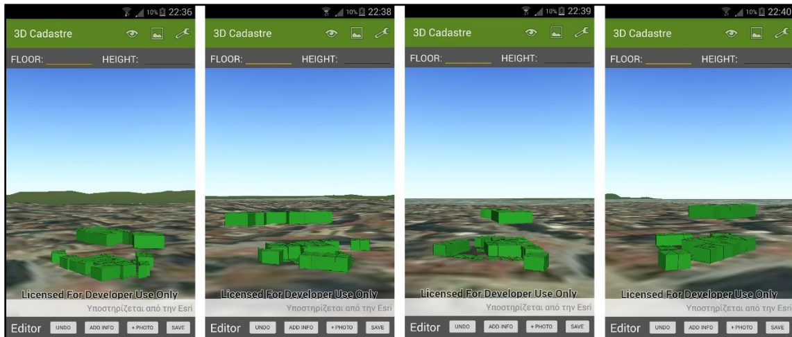
Figure 117. 3D Visualization of the declared properties (in green) in their absolute position on the ground, using the 3D View tool of the mobile application.
