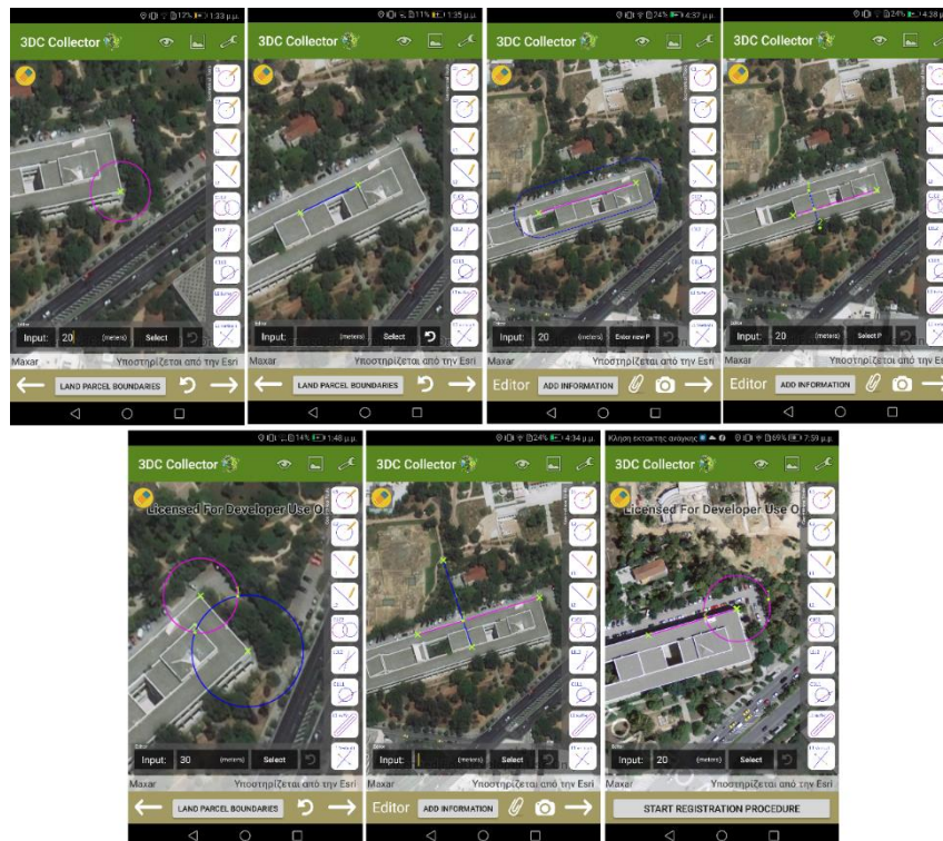
Figure 91. Geometrical drawing tools offered by BoundGeometry application. Top (left to right): circle, line, offset to line, vertical lines Bottom: intersection points between 2 circles, 2 lines, a circle and a line.
