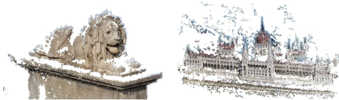
Figure 64. Reconstruction from smart phone images (left), Dense point cloud of the Parliament building after reconstruction from images (right) (Source: Somogyi et al., 2016).
