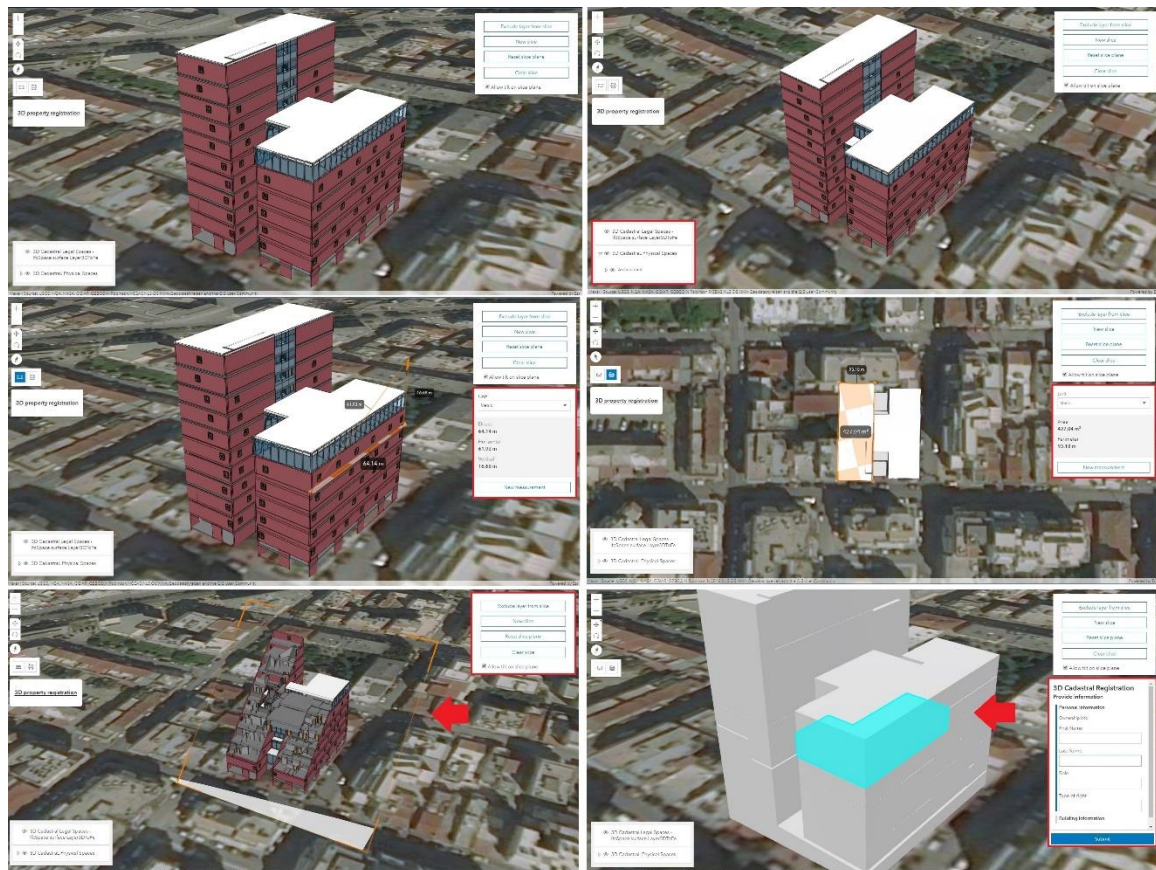
Figure 97. Top row (left to right): the application’s interface and the layer management tool. Middle row (left to right) the 3D length measurement tool and the 3D area and perimeter measurement tool. Bottom row (left to right): the building slicing tool and the editor tool.
