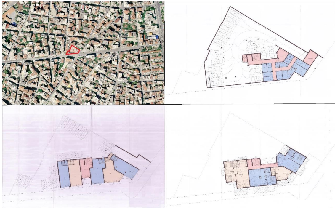
Figure 115. Orthophoto of the case-study area at the scale of 1:1000 (top left) and the floor plans of the underground floor (top right), the ground floor (bottom left), and third floor (bottom right) at the scale of 1:50.
