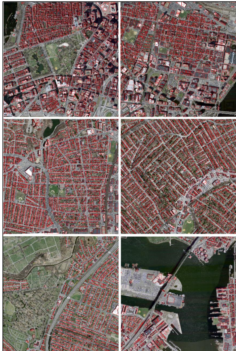
Figure 55. Example of the detected buildings in vector format, overlaid to an orthophoto depicting the respective study area.
