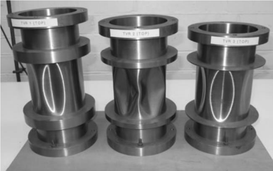
Figure 1.7: Shell instability of thin-walled circular cylinders under external pressure. [Ross, 2011]
