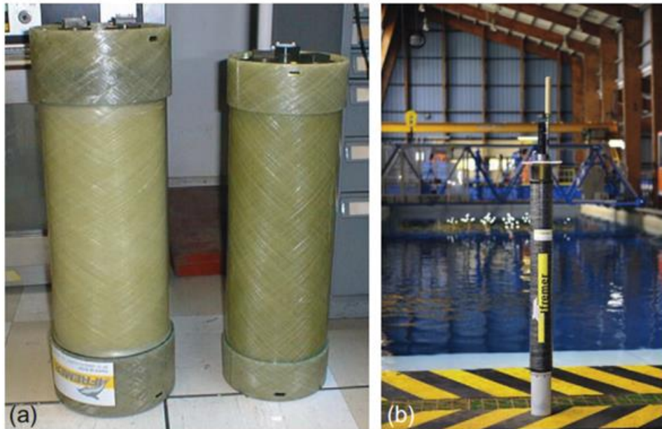
Figure 1.6: Oceanographic instrument protection casings (a) Glass/epoxy filament wound housings (500mm long, 150mm inner diameter) (b) Deep Arbor profiler engaged in ARGO project (1000mm long, 100mm inner diameter) [Davies, 2016]
