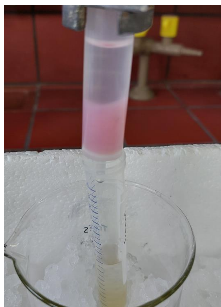
Figure 2.8: The IMAC chromatography column for the purification of recombinant proteins
