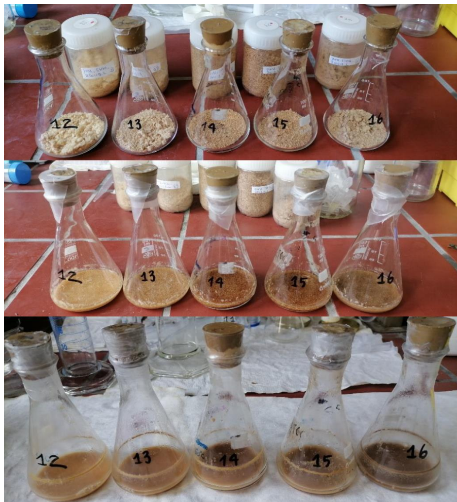
Figure 2.3: The enzymatic hydrolysis experiment. Top to bottom: lignocellulosic biomass in the flasks, the biomass-Cellic Ctec2 ® mixture at the start of the hydrolysis, the mixture after the hydrolysis
