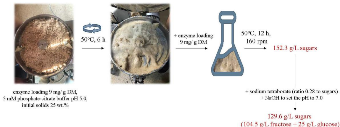
Figure 3.4: Overall scheme of scale-up reaction towards the production of a fructose-rich syrup.
