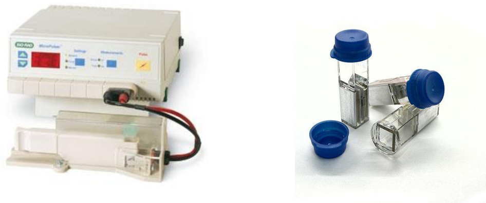
Figure 2.6: Electroporator and cuvettes used in the electroporation experiments.
