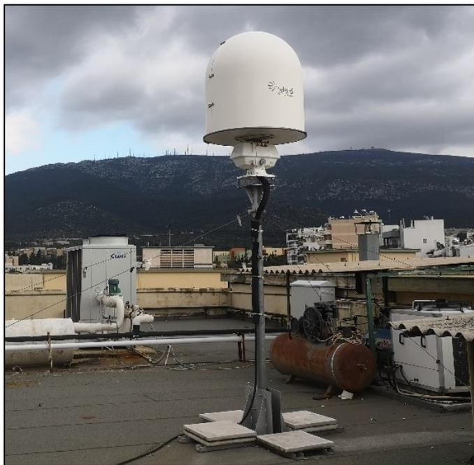
Figure 2-6: The installed Rainscanner® unit, Antenna and Head unit
