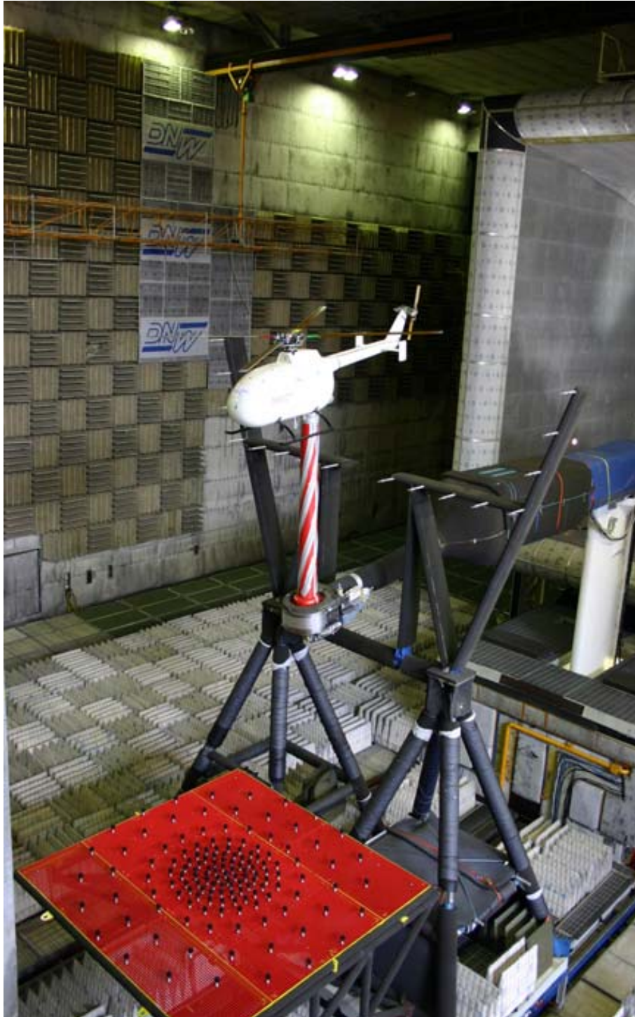
Figure 3.17. BO105 helicopter wind tunnel model used in the HeliNoVi experimental campaign. Image copied from [10].
