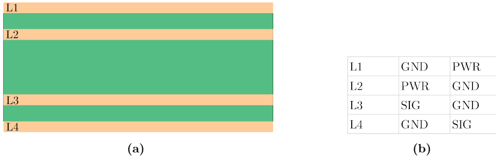
Figure 2.10 Layer order recommendations for a 4-layer board.
