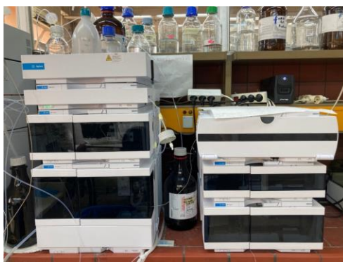
Figure 23. Agilent 1260 Infinity II instrument
