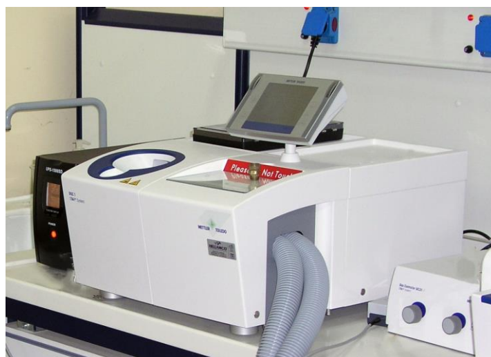
Figure 24. Mettler DSC 1 STARe System
