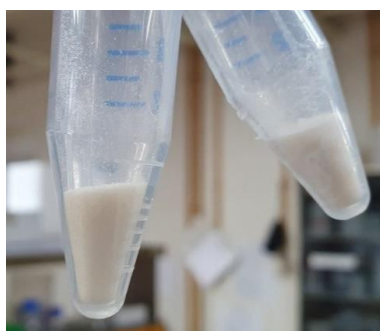
Figure 60. Immobilized on the EziG3 Amber carrier LCC ICCG
