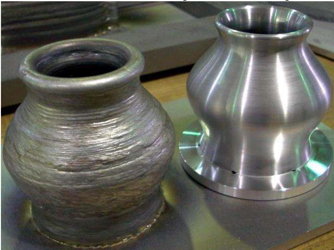
Electron Beam Free Form Forming. Pre and Post Machining
