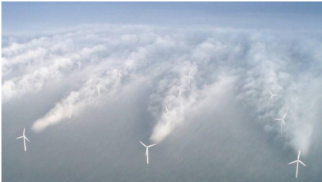
Figure 4: Wake turbulence Vattenfall Wind Power, Denmark [25]
