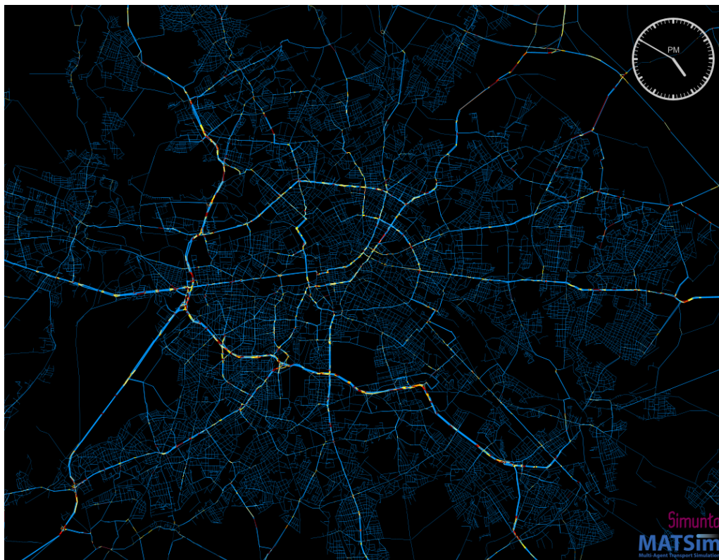
Figure 53: Scenario 3c - traffic volumes and congestion points at peak hours: 16:50 (links colors/width as above)
