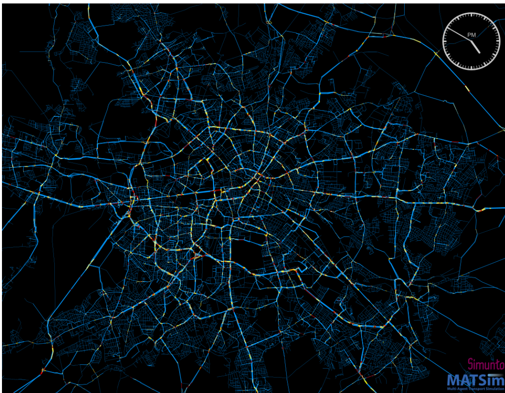
Figure 49: Scenario 2b - traffic volumes and congestion points at peak hours: 16:50 (links colors/width as above)
