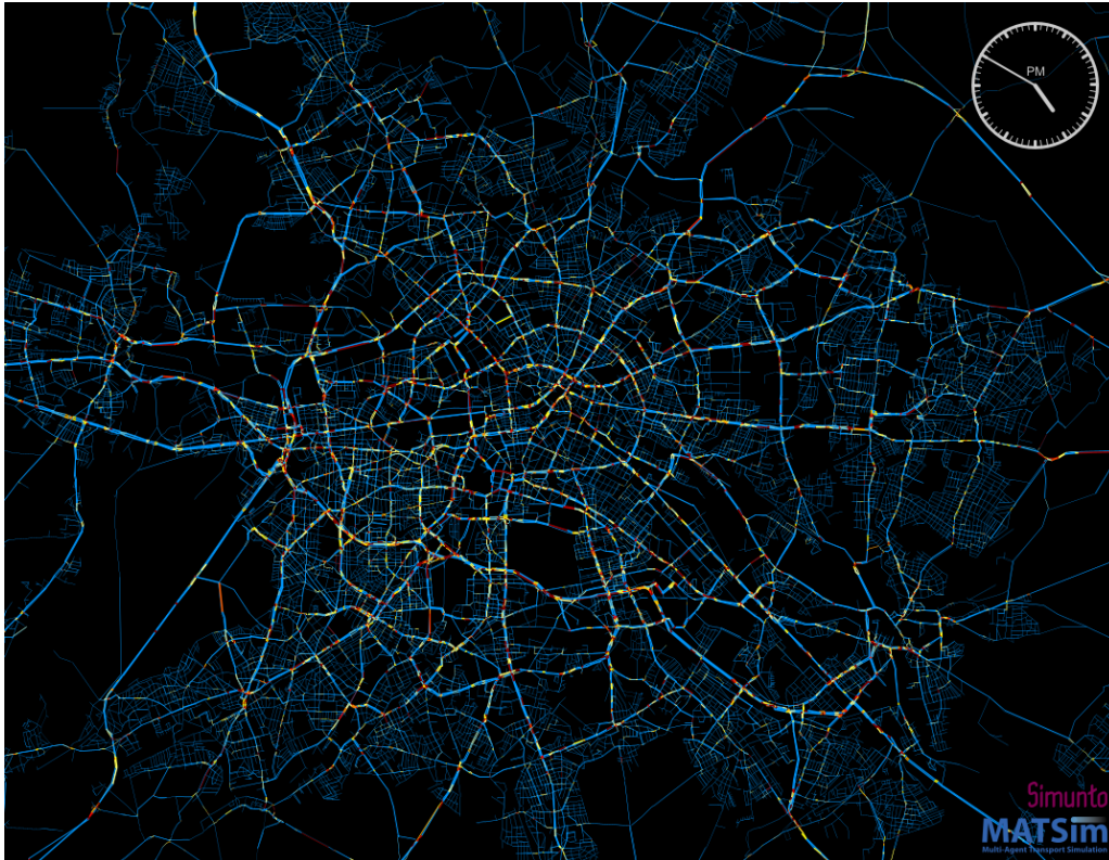
Figure 48: Scenario 2a - traffic volumes and congestion points at peak hours 16:50 (links colors/width as above)
