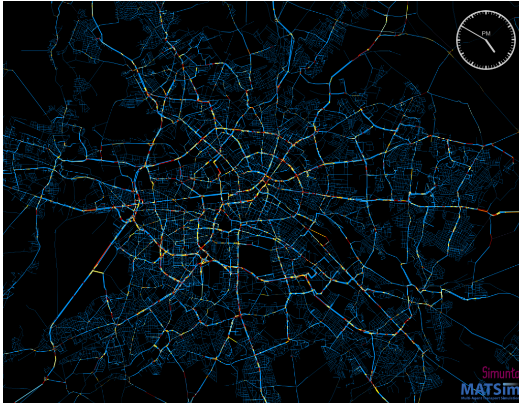
Figure 50: Scenario 2c - traffic volumes and congestion points at peak hours: 16:50 (links colors/width as above)
