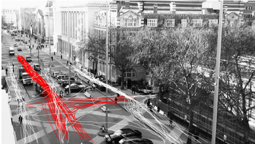
Figure 9: Trajectories in Exhibition Road, London, UK, pedestrians with white and vehicles with red. Source: (Anvari et al., 2016)
