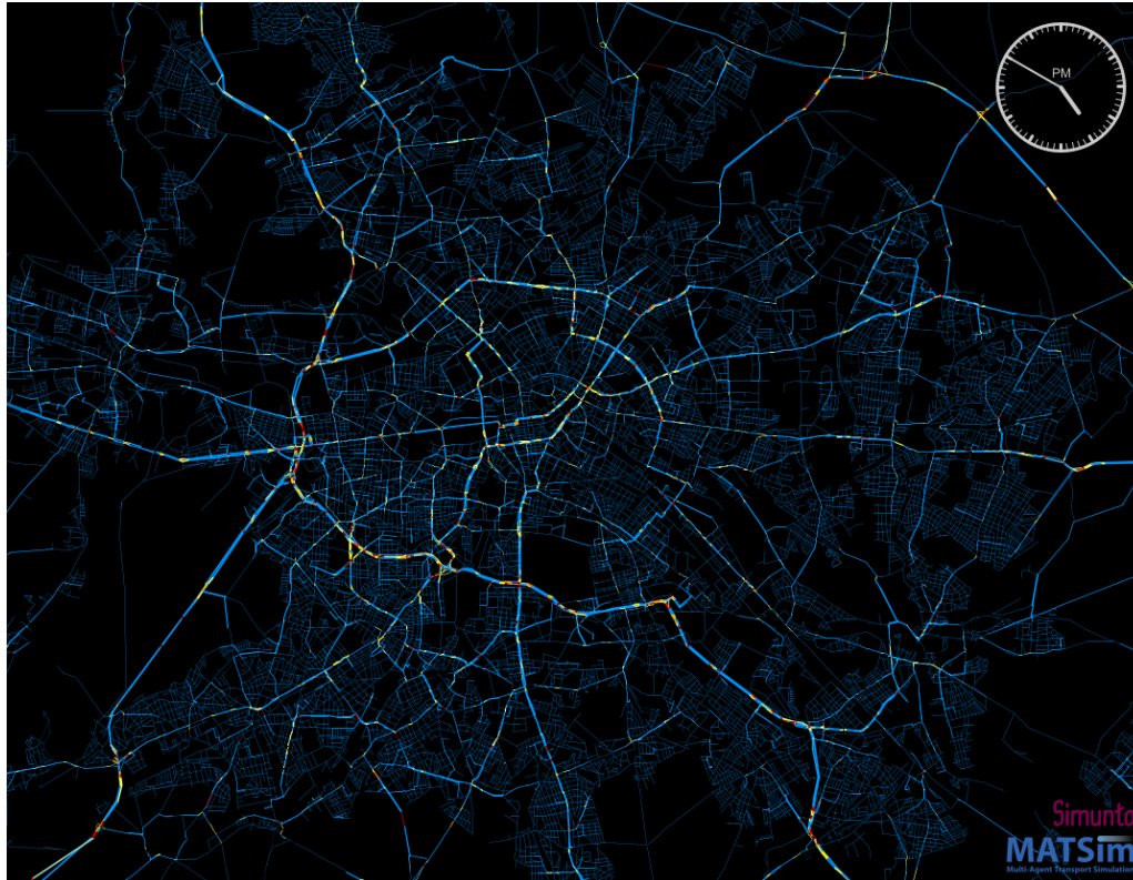
Figure 52: Scenario 3b - traffic volumes and congestion points at peak hours: 16:50 (links colors/width as above)
