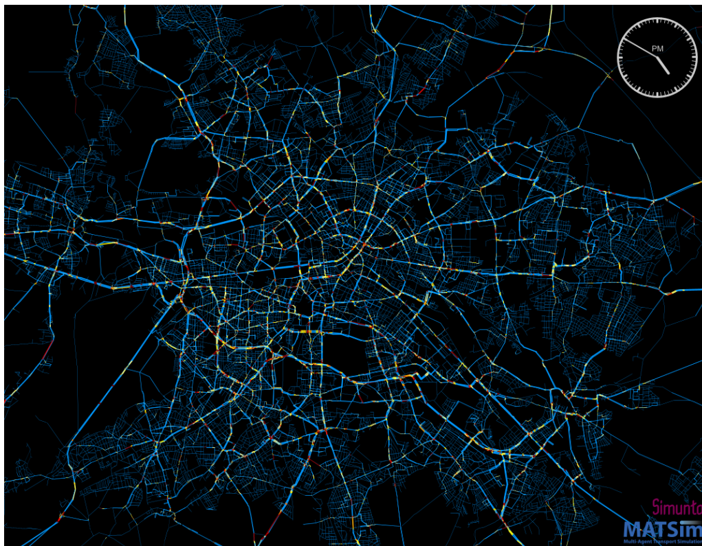
Figure 51: Scenario 3a - traffic volumes and congestion points at peak hours: 16:50 (links colors/width as above)
