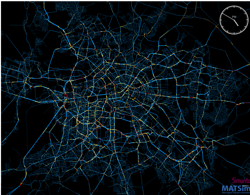
Figure 47: Scenario 1b - traffic volumes and congestion points at peak hour: 16:50, i.e., the link width is related to the traffic volume; links with dark red: rel = \frac{u_{ac}}{u_f} \leq 0.85 , with red: rel \leq 0.875 ; with orange: rel \leq 0.90 , with yellow: rel \leq 0.925 , with light yellow: rel \leq 0.95 and blue: rel > 0.95 .
