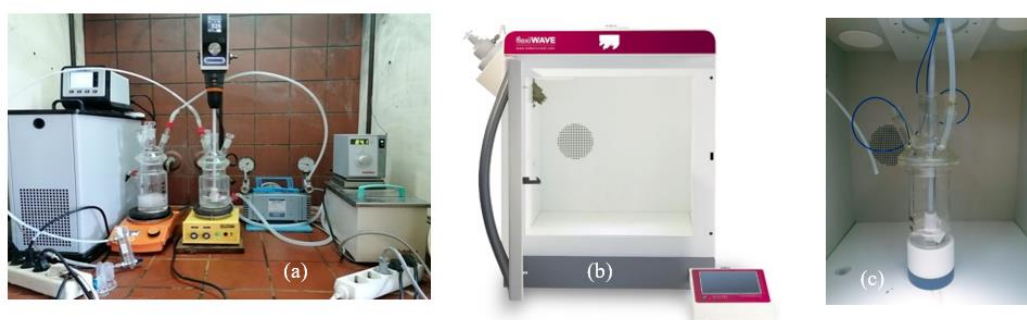
Figure 4.1. Picture of the experimental reactor setup used for the study (a) Conventional Synthesis: jacketed reactors connected with oil/water bath, vacuum pump, overhead stirrer 29 , (b) flexiWAVE MW Synthesis Platform, (c) internal of MW cavity with glass reactor.
