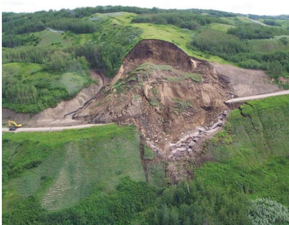
A translatational landslide that occurred in 2001 in the Beatton River Valley, British Columbia, Canada. (Photograph by Réjean Couture, Canada Geological Survey.)
