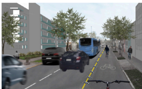
(d) Bike lane marked with a line and physical barriers
