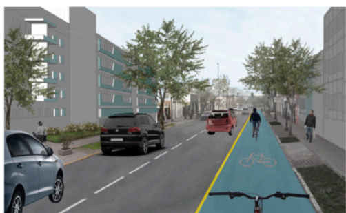
(c) Bike lane marked with painted surface
