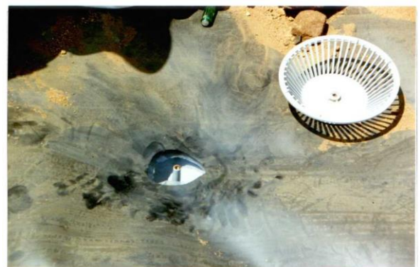
Photo 11. The installation of water collection system at the bottom of lysimeters.
