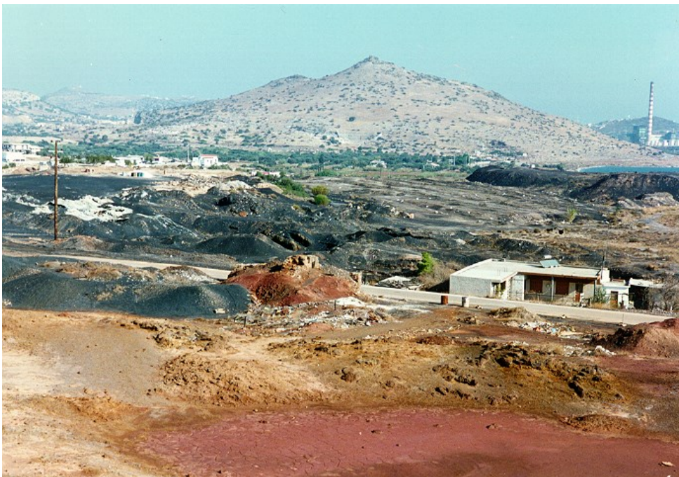
Fig. 4. Metallurgical processing wastes at Kavodokanos-Thorikon in Lavrion. In the foreground pyritiferous tailings (red to yellow-brown) on which the demonstration scale rehabilitation techniques were applied, and in the central part lumpy and pelletised slag, and sand-blast wastes (black to grey-black).
