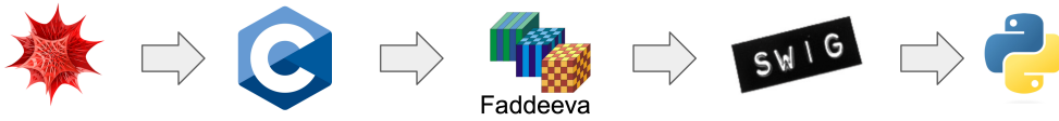
Figure 2.1: Workflow for transforming an analytic expression obtained initially in Mathematica to a Python library.
