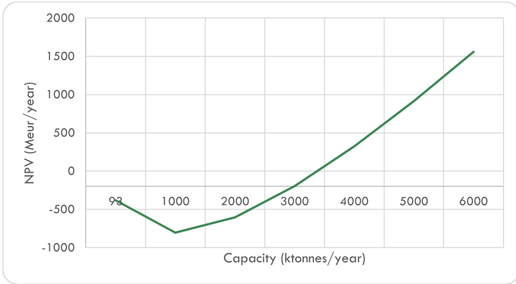
Figure 22: The evolution of NPV as a function of capacity, with the method of economy of scale, for the second case study, in year 2050, and for a methanol price of 1720 eur/tonne.
