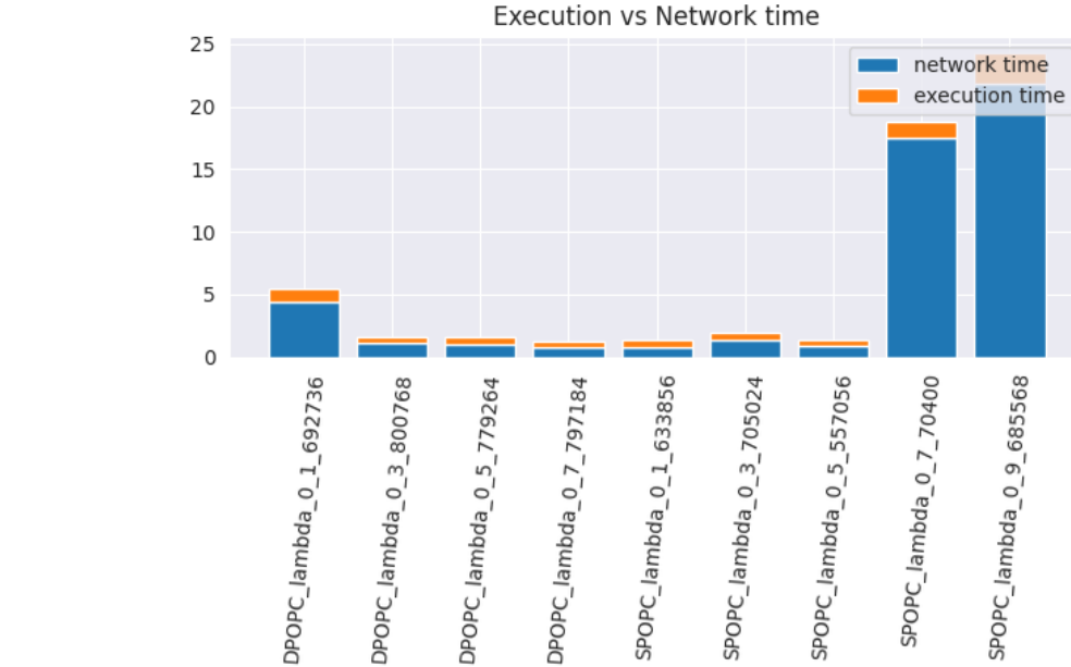
Figure 5.3.14: Execution vs Network time in layered execution for \lambda_{max} = 25 and num\_clients = 1
