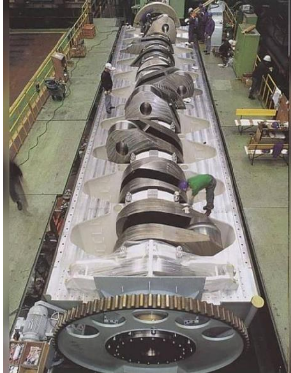
Figure 6: Crankshaft of a Two-Stroke Marine Engine
