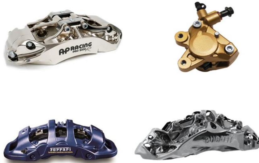
Figure 3 Different brake caliper designs. U. Left: AP Racing PRO 5000, U. Right: Yamaha R1 piston caliper, L. Left: Ferrari racing brake caliper by Brembo, L. Right: Bugatti 3D printed caliper
