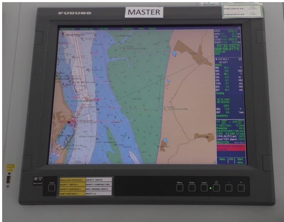
Figure 5: An ECDIS display on a cargo vessel. Author's image.
