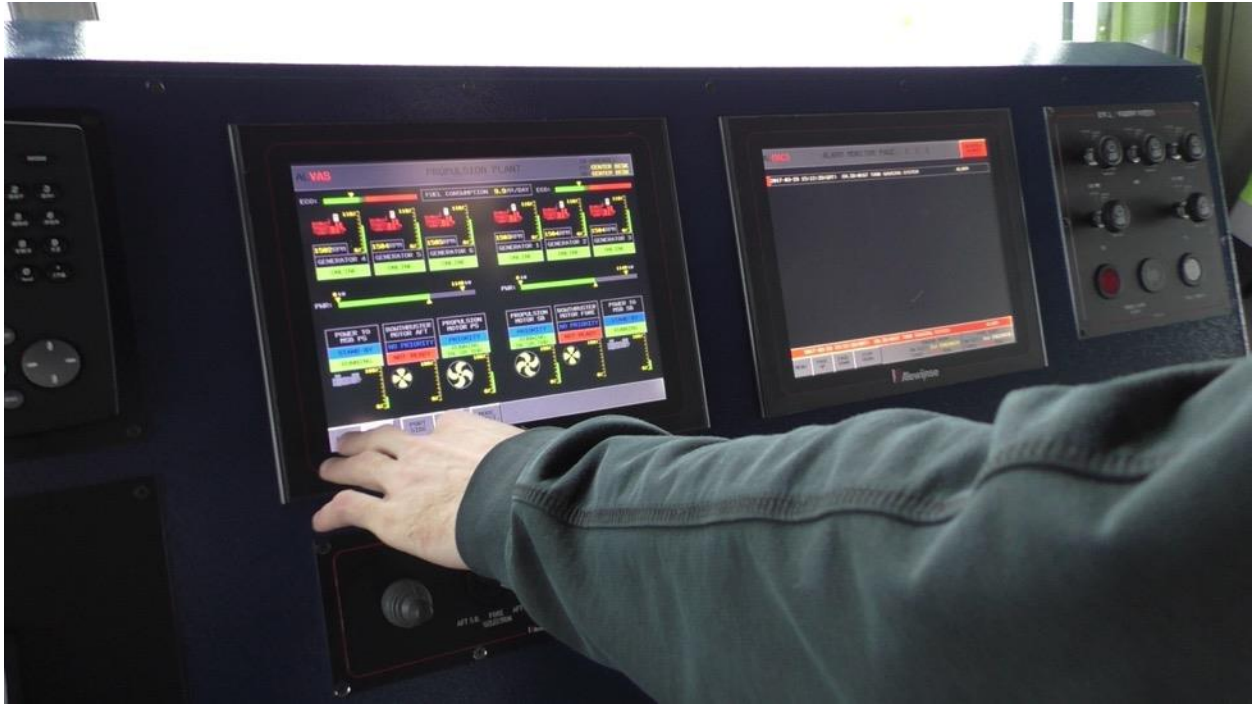
Figure 35 EMS DUNDEE: The officer on watch during the tour of the ship bridge instruments. The MFD for the interface of the engine system is turned on in the propulsion control mode. Author's image.
