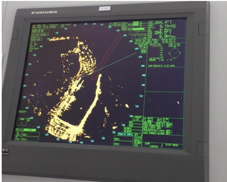
Figure 4: An X-band RADAR system on a cargo vessel. Author's image.
