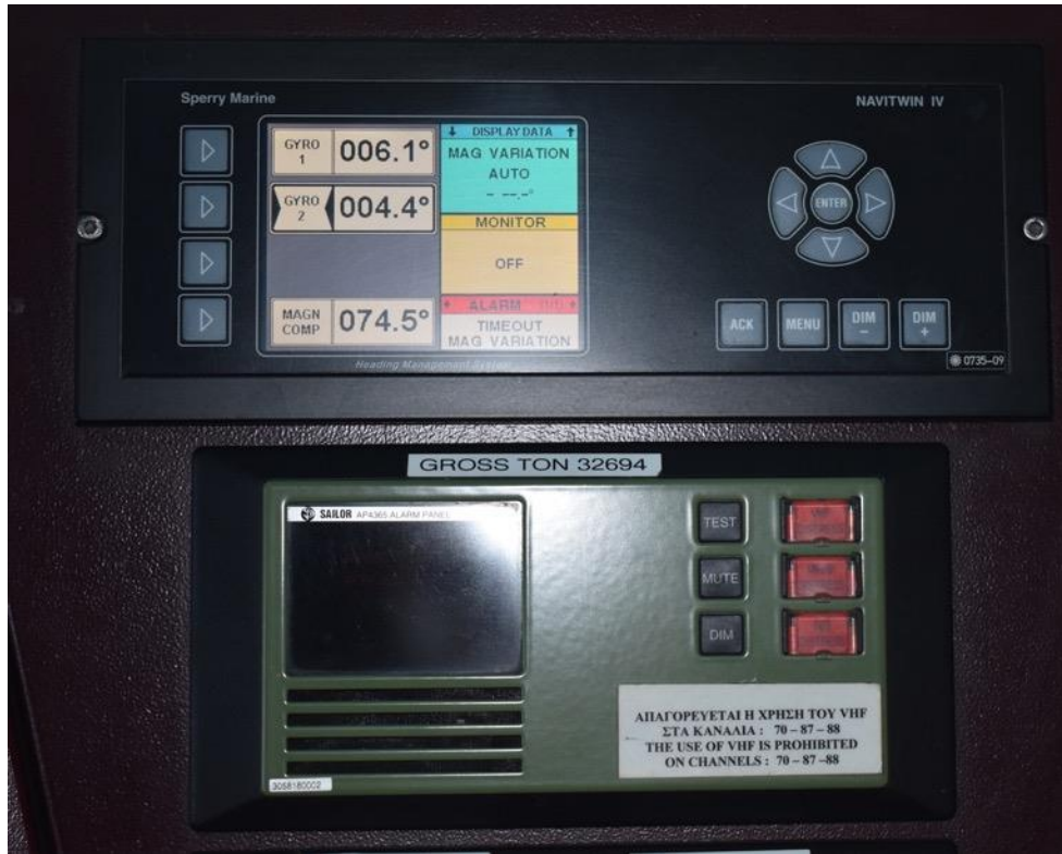
Figure 8: A heading management system display (top) and a Global Maritime Distress and Safety System (GMDSS) panel (bottom) of a Ro-Ro/Passenger Ship. Author's image.
