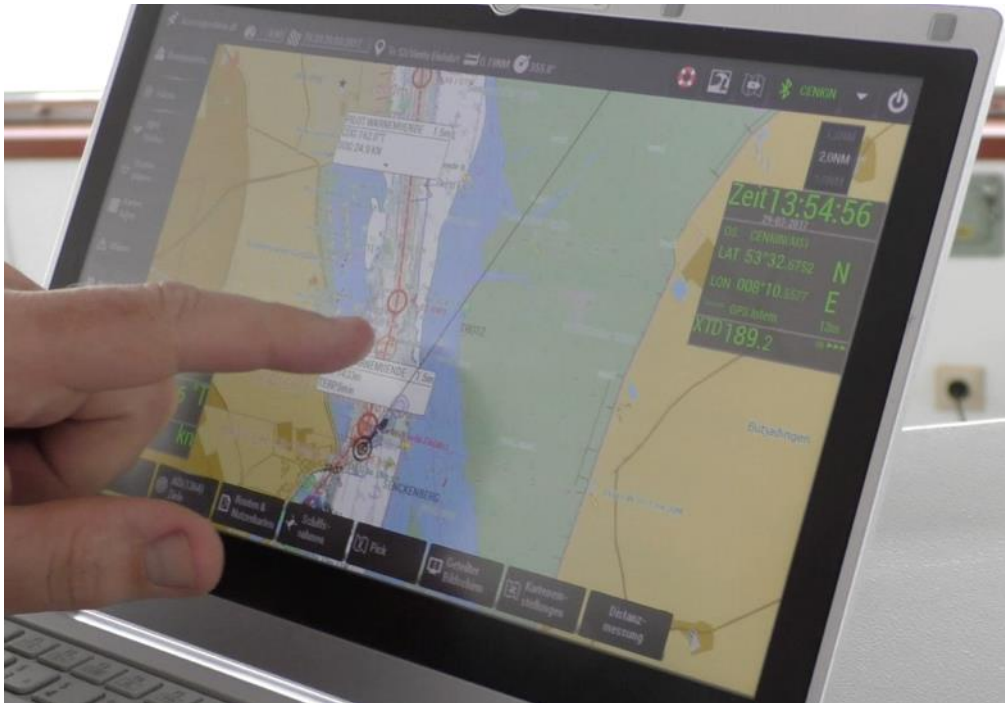
Figure 36 The pilot explains how the PPU can be used to observe other ships' courses. The meeting points on the display indicate passing and overtaking manoeuvres. Author's image.
