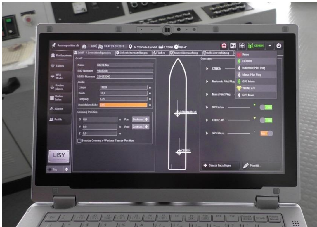
Figure 14: A Portable Pilot Unit in operation on board a cargo vessel. Author's image.
