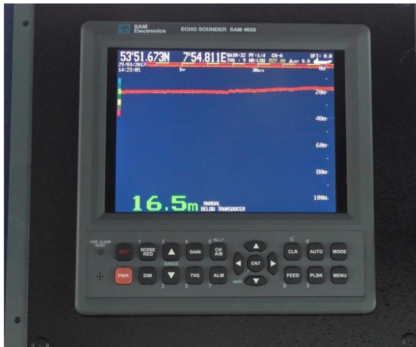
Figure 9: An echo sounder on a cargo ship. Author's image.
