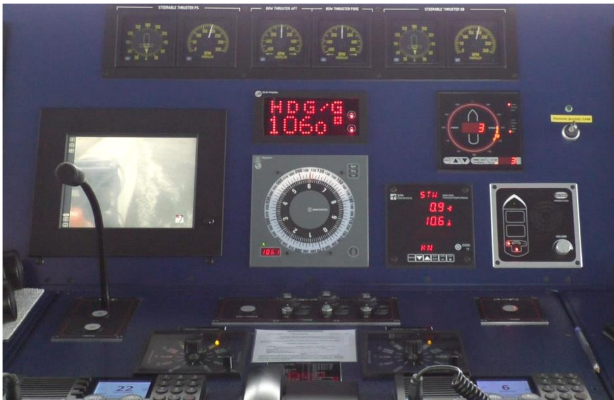
Figure 11: Various instruments on a ship bridge. Thruster indicators (top), camera view from starboard side (middle left), gyrocompass (middle bottom) and heading (middle top), wind direction and speed (middle right), vessel speed and microphone (bottom right).
