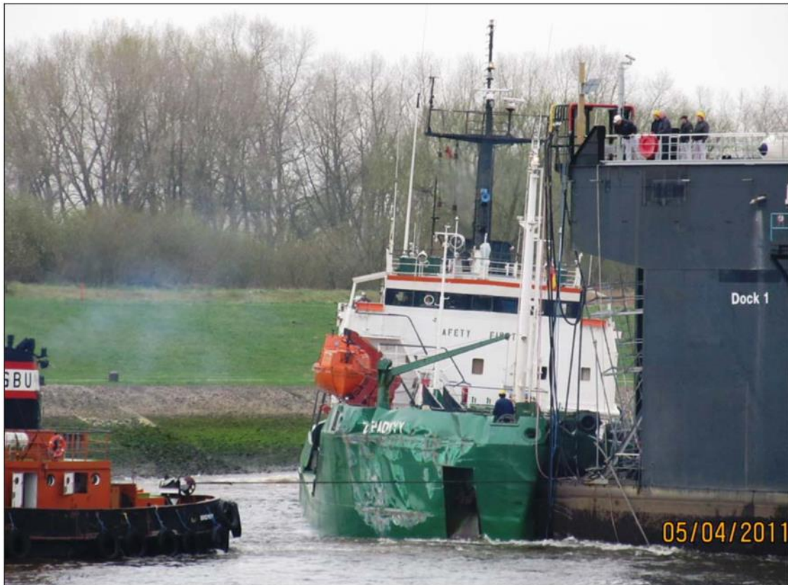
Figure 2: Front end of floating dock wedged into forecandle of the ZAPADNYY. A tug boat is depicted during the effort to release the ZAPADNYY from the dock (BSU, 2012).
