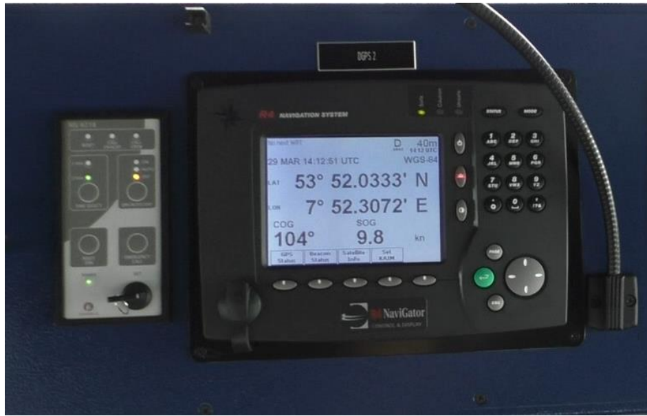
Figure 10: A DGPS display on board a cargo vessel. Author's image.
