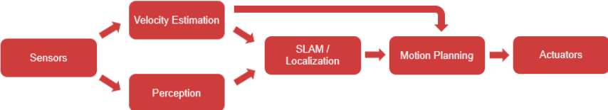
Figure 3.7: The autonomous system software pipeline.
