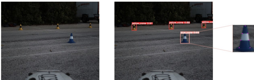
Figure 5.3: The perception pipeline with the keypoint network added.
