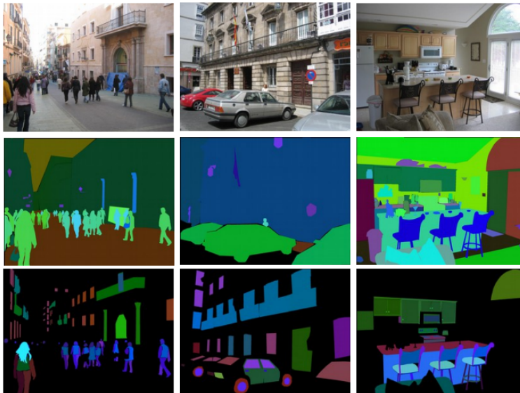
Figure 1.2.2: Annotations in ADE20k. Second row has object annotations and third row has object parts annotations.
