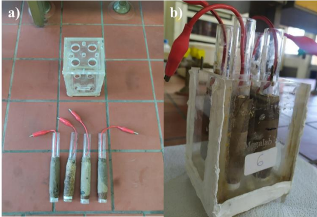
Figure 10. Rectangular Plexiglas single chamber air cathode MFC. a) Disassembled cell and b) Assembled cell with Gore-Tex electrodes during leakage test.
