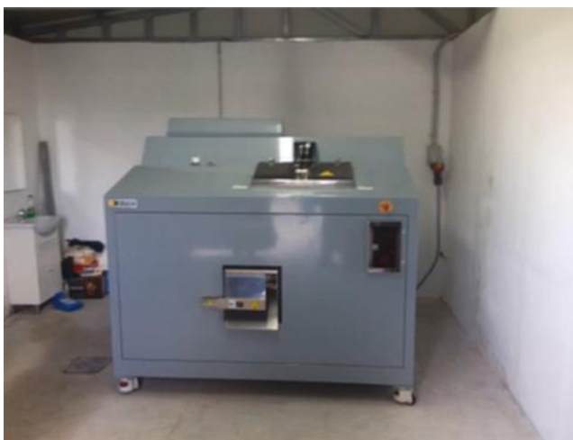
Figure 22. Shredder, dryer and condenser used for the exploitation of HFW in Halandri, Athens, Greece.
