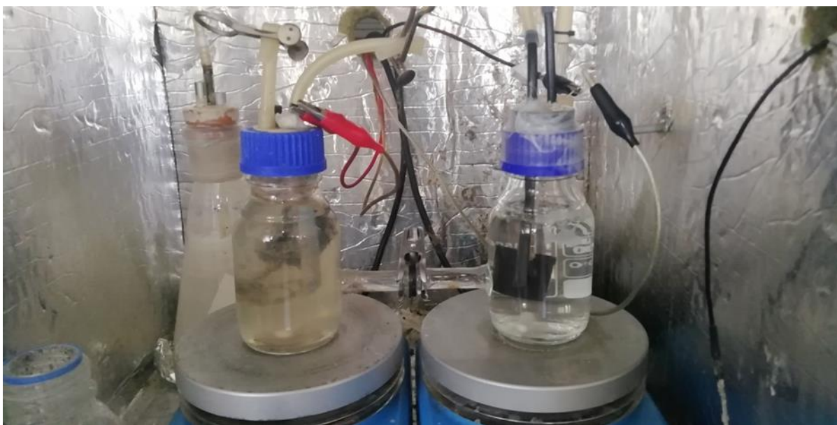
Figure 19. Glass dual chamber MFC, operating with oxygen (air pump – black tube) as the electron acceptor, during acclimation.
