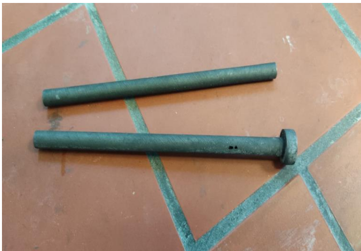
Figure 14. Graphite rods used to facilitate the current collection from the graphite granule bed.
