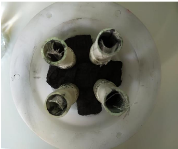
Figure 15. Stainless steel sponges placed in a cylindrical single chamber air cathode MFC with 4 mullite electrodes.
