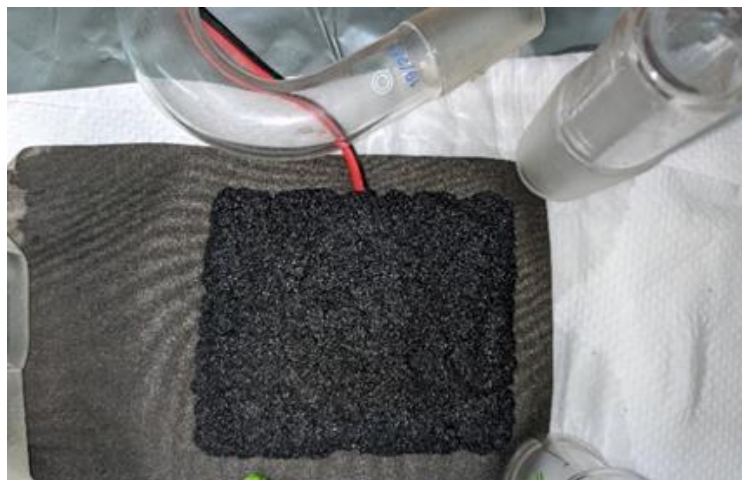
Figure 16. Oxygen reduction catalytic paste spread on a Gore-Tex cloth with a copper wire inserted for electron collection.
