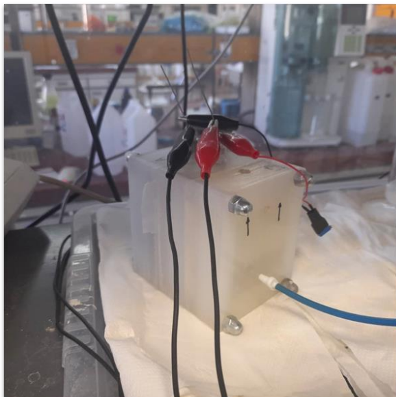
Figure 20. PTFE dual chamber MFC, operating with oxygen (air pump – blue tube) as the electron acceptor, during acclimation.
