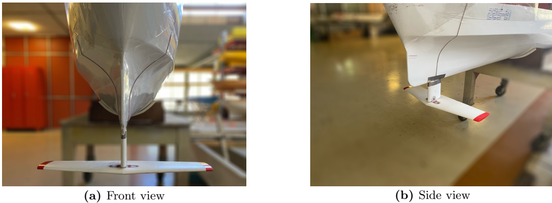
Figure 6.1: Pictures of the experimental arrangement of a reverse T-foil placed in under the bow of scaled ferry ship. Ship dimensions: length L=3.3\text{m} , breadth B=0.43 and draught T=0.135\text{m} . Foil dimensions: span s=0.5\text{m} , sweep angle \theta = 12^\circ
