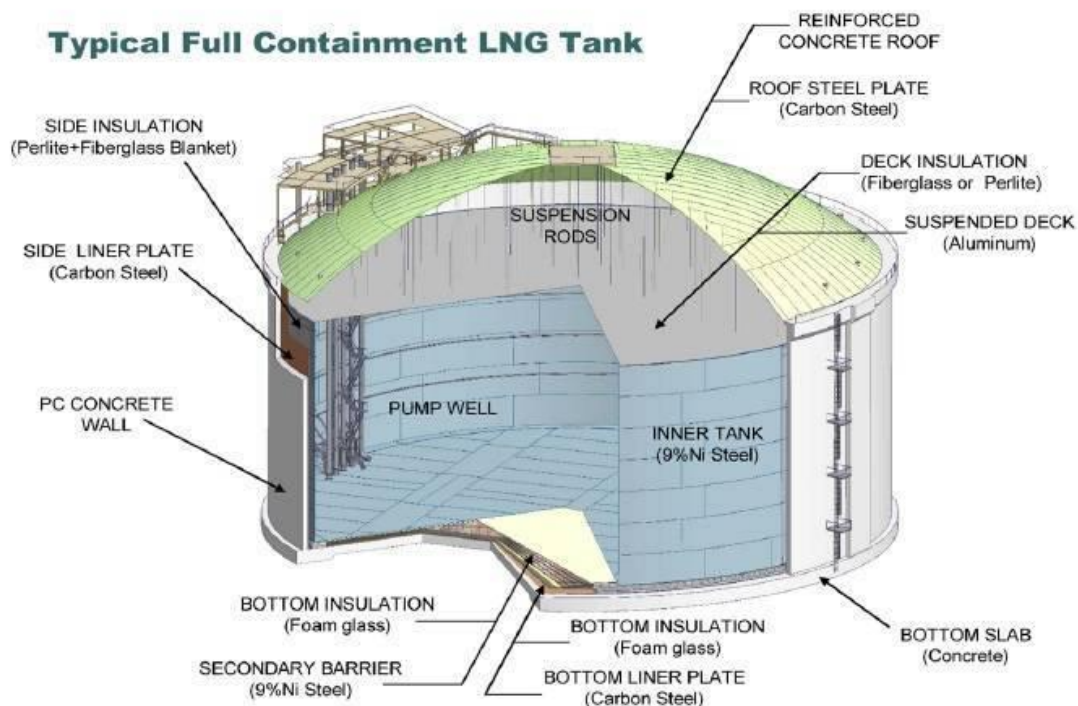
Figure 3-2: LNG cryogenic storage at shore.
