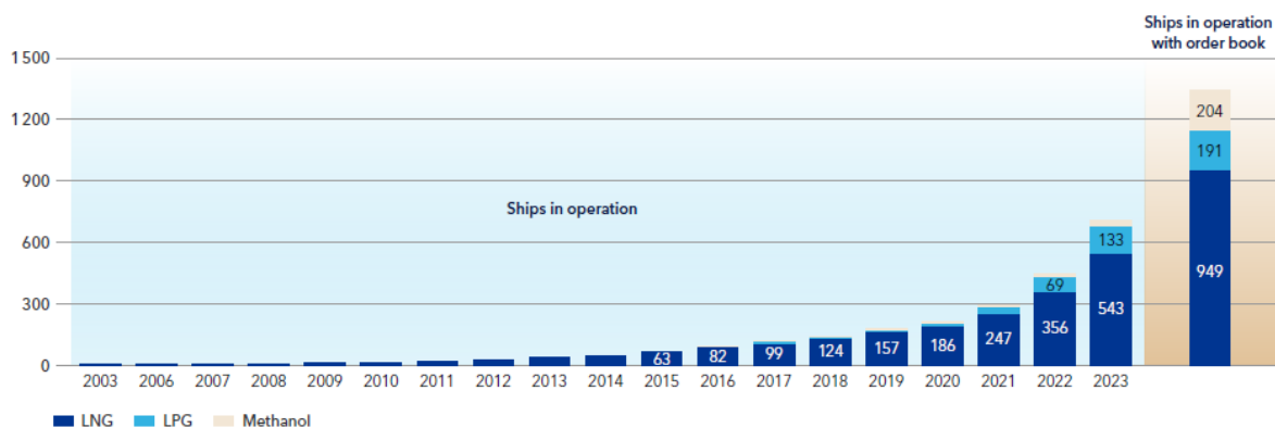
Figure 6-2: Development of LNG, LPG and methanol fuel technology uptake by number of ships, excluding gas carriers. (DNV)
