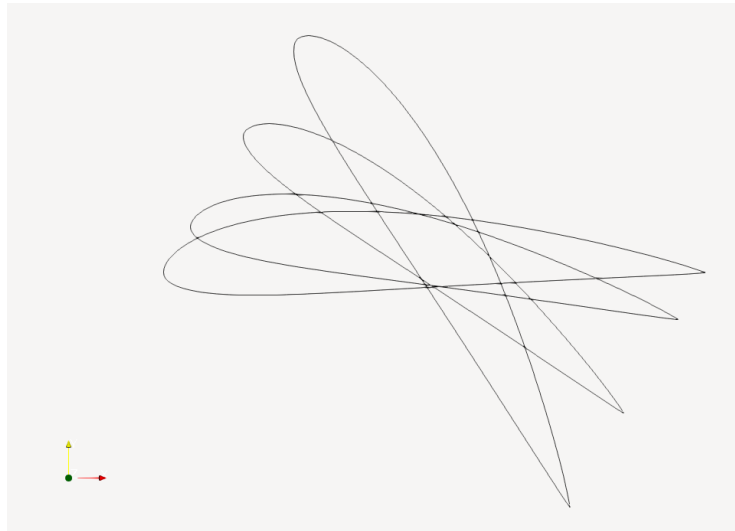
Figure 2.2: Example of displacement of the NACA4415 Airfoil using the Sub-Step Displacement Method. The airfoil is rotated and the total displacement has been achieved in 3 sub-steps.
