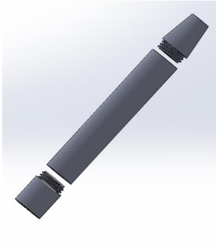
Figure 2.7: The second solution with the thread connection of the parts of the device
