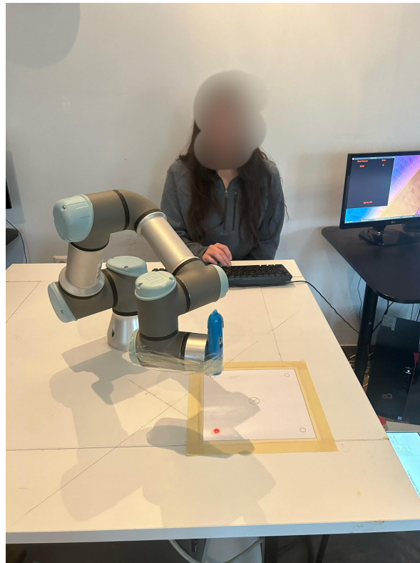
Figure 5.6: The Human-Robot Collaboration setup The robot is placed in the middle of 1m x 1m table.
