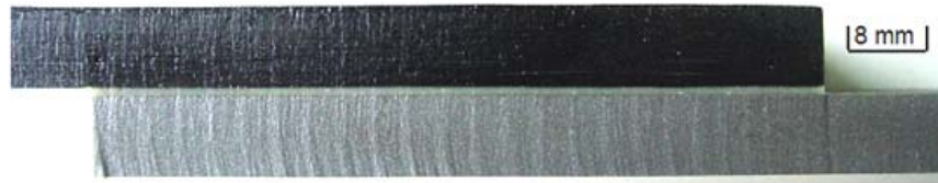
Figure 7.3: Side view of a typical SLJ with 75 mm overlap length.
