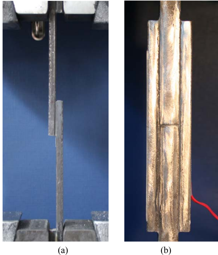
Figure 6.2: Experimental test of (a) a SLJ and (b) a DSJ specimen.
