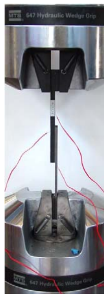
Figure 7.5: A typical CFRP-to-Steel SLJ with 75mm overlap length under experimental conditions.
