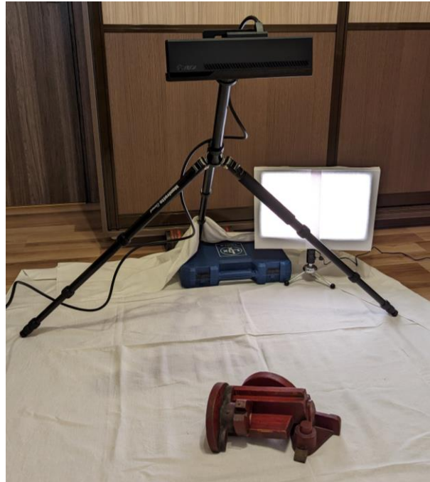
Figure 6-20: Camera setup for acquiring images.
