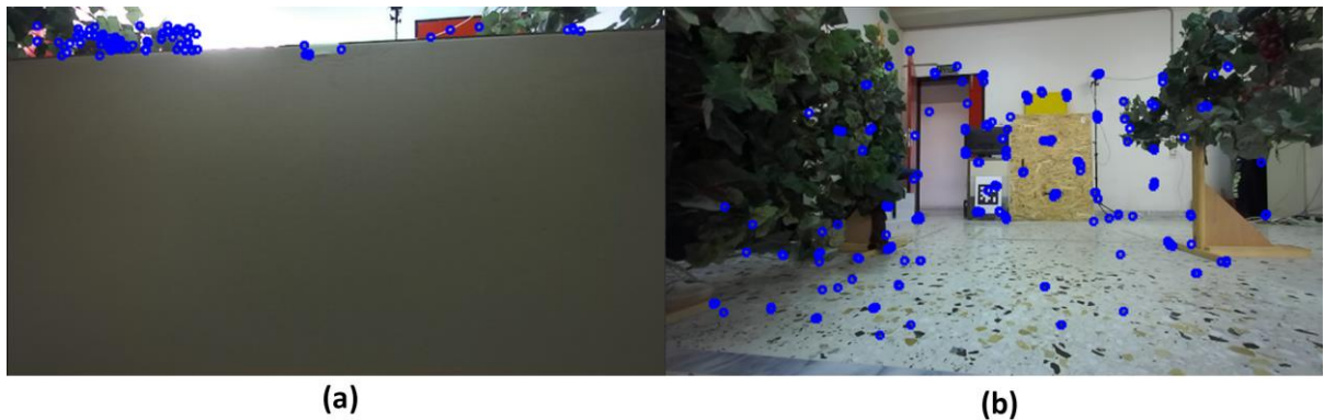
Figure 3-5: (a) One camera's lenses are obstructed resulting in very low number of detected features. (b) A different camera is not obstructed and continues to produce accurate visual odometry [17].
