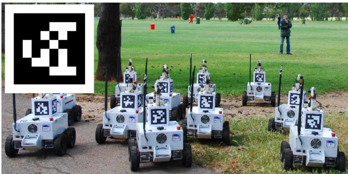
Figure 3-6: April Tags used for research purposes in April Laboratory, University of Michigan [69].
