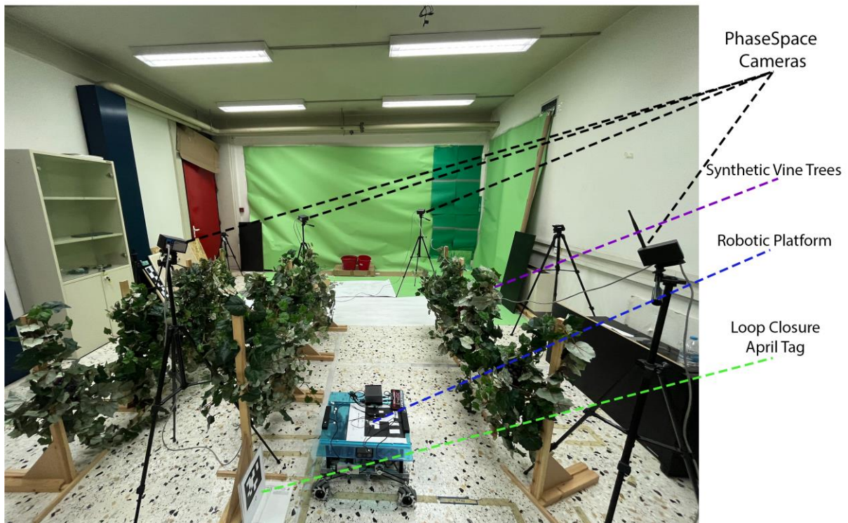
Figure 7-3: Indoor testing environment with artificial lighting and PhaseSpace system.
