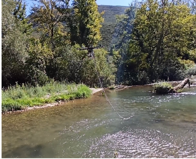
FIGURE 2.6: The octorotor with the cable-suspended sampling mechanism during the sampling procedure in a river.
