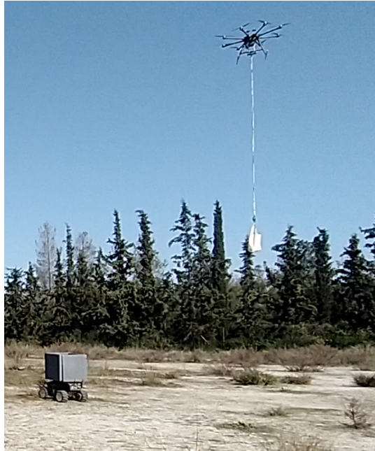
FIGURE 4.1: The multirotor with the cable-suspended load and the UGV deployed in the field.
