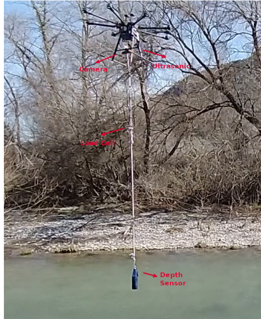
FIGURE 5.3: The position of the additional sensors required during the water sampling procedure.
