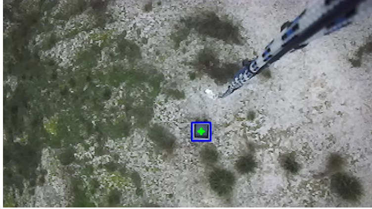
FIGURE 4.3: Detection of the target. The green cross corresponds to the center of the bounding box.
