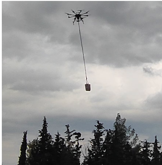
FIGURE 3.1: The octorotor with the cable-suspended load deployed in the field.
