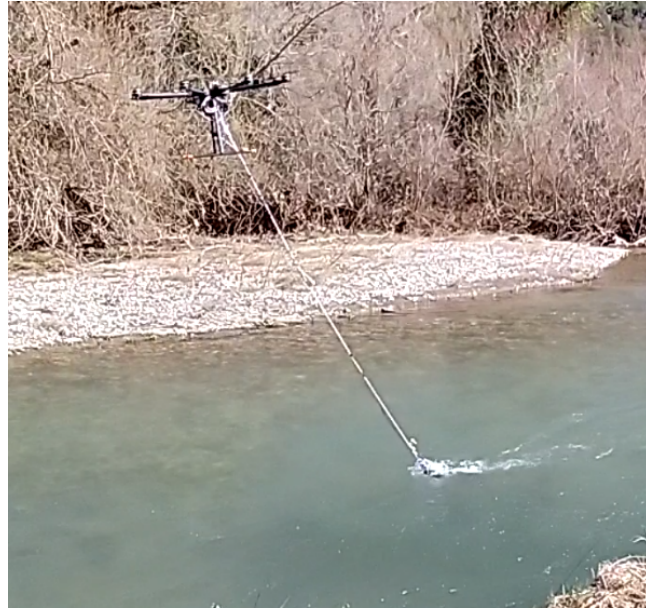
FIGURE 5.1: Water Sampling with an octorotor in a river.
