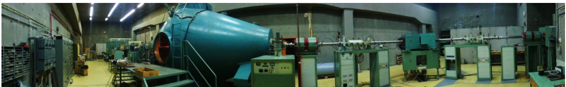
Figure 3.6: The 5.5 MV Van de Graaff accelerator of the “Demokritos” facility
