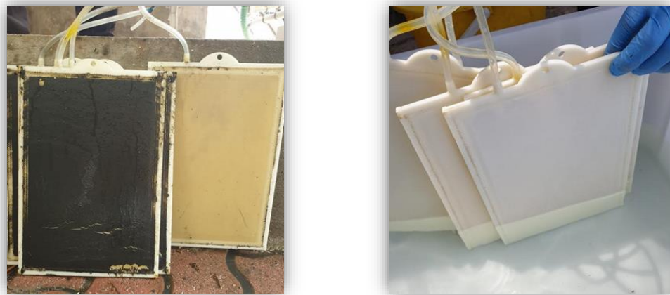
Figure 4. 42: Flat sheet membranes before (left) and after(right) chemical cleaning.
