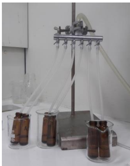
Figure 3. 7:solvent evaporation using nitrogen gas, immediately after the collection of the eluates in dark-colored vials from solid-phase extraction
