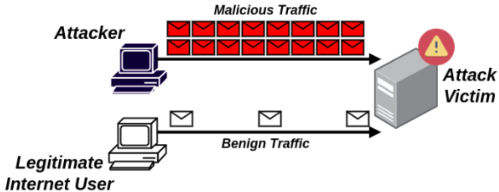
Figure 2.6: Denial of Service (DoS) Attacks - The attacker floods the victim with superfluous Internet traffic to disrupt legitimate Internet users from using online services
