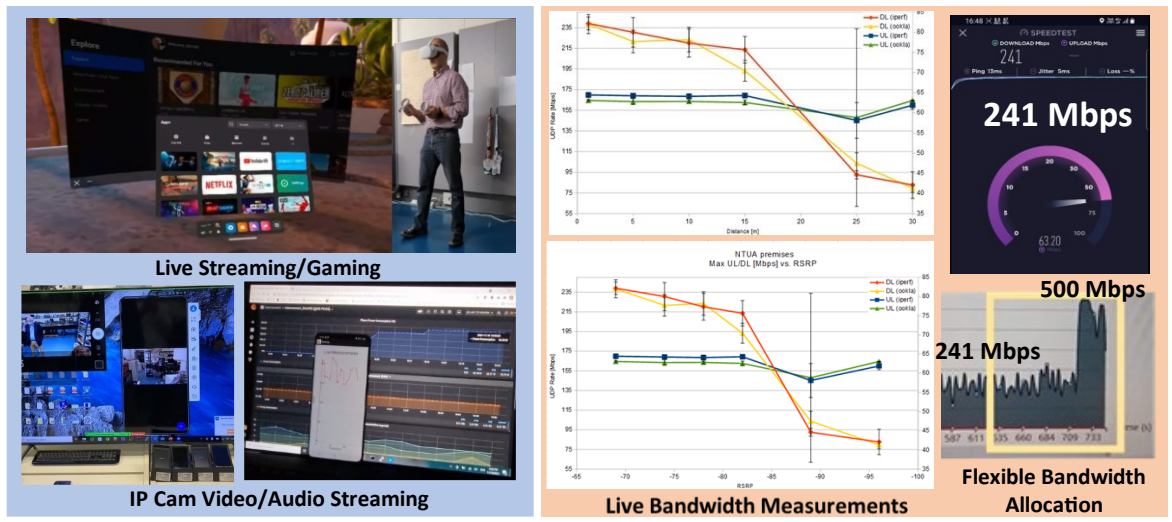
Figure 50. Service/Control layer evaluation of analog TxRx interface, including: Dynamic capacity reconfiguration, Live latency/bandwidth measurements, Live Bandwidth measurements, and Demonstration of the uninterrupted operation of AR/VR gaming, 4K video streaming, and IP videos, over the presented deployment.
