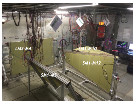
Figure 4.39: The Micromegas high voltage validation experimental setup at BB5.
