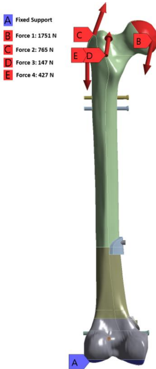
Figure 87: FEM Boundary Conditions for the 80kg benchmark weight
