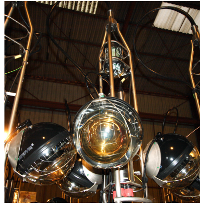
Figure 2.8: A storey with the three optical modules attached. Image credit: [15]
