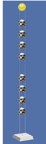
Figure 2.3: A schematic representation of a Detection Unit (DU). Image credit: [8].
