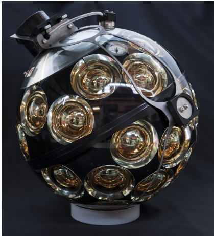
Figure 2.1: Digital optical module (DOM). Image credit [8].
