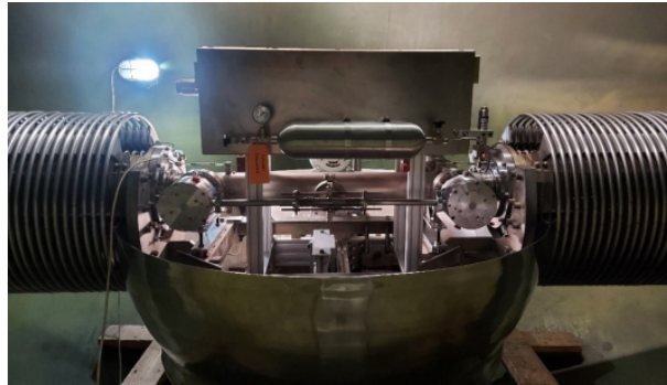
Figure 2.2: The new stripping canal in the accelerator tank [29]
