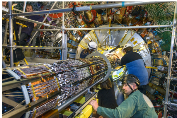
Figure 2.12: The pixel detector, the innermost component of the ATLAS inner detector, featuring layers of high-resolution silicon pixels. It provides precise measurements of particle positions near the collision point, essential for identifying primary and secondary vertices [33].
