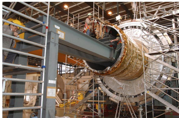
Figure 2.8: The central solenoid magnet of the ATLAS detector, responsible for generating a strong and uniform magnetic field that bends the paths of charged particles within the inner detector, enabling precise momentum measurements [29].
