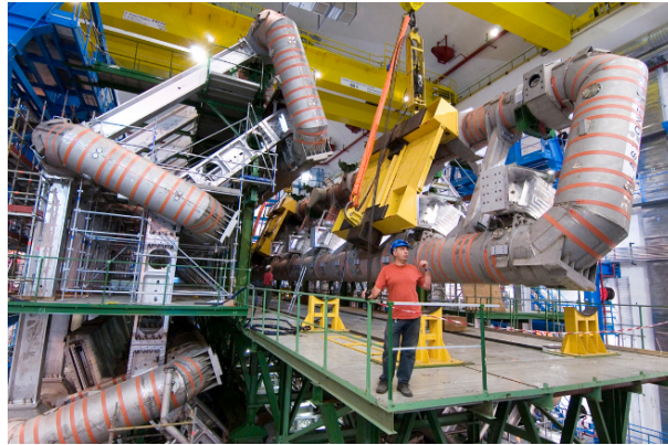
Figure 2.9: The barrel toroid magnet of the ATLAS detector, a large superconducting magnet that surrounds the calorimeters, producing a magnetic field that bends the paths of charged particles in the outer regions of the detector, essential for momentum measurements of particles emerging from high-energy collisions [29].
