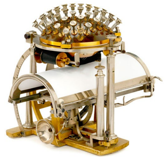
The Hansen Writing Ball (this model dates from c. 1875) was an early version of the typewriter developed by Rasmus Malling-Hansen in 1865.
