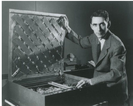
Shannon is posing with a maze he built for an electronic mouse, named Theseus
