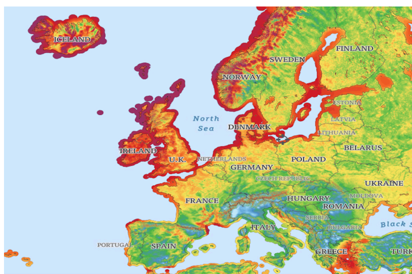
Figure 5.6: Average wind speeds in Europe. The red color indicates higher speeds (Global Wind Atlas).
