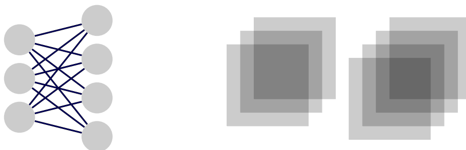
Figure 3.1: DNNs operate using nodes and CNNs operate using channels. A DNN layer takes 3 nodes and returns 4 nodes (left), while a CNN layer takes 3 channels and returns 4 channels (right).
