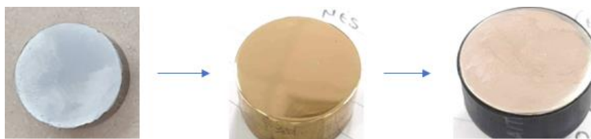
Figure 48: Samples before (left) the pre-treatment , after (middle) the pre-treatment, after (right) the electrodeposition
