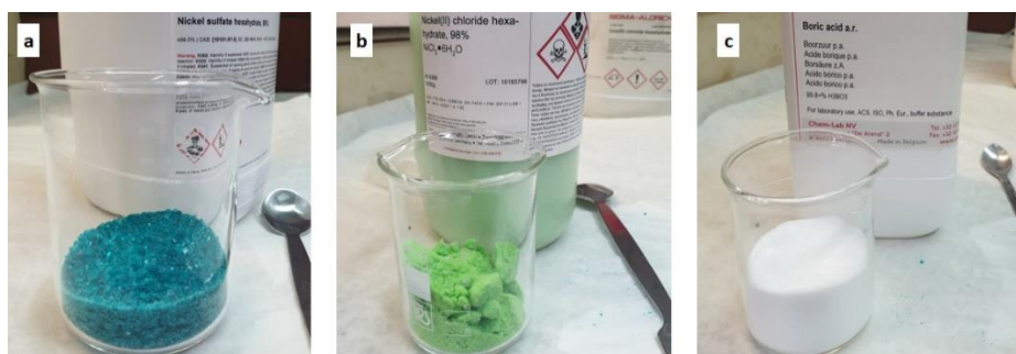
Figure 49: Ni-Watts electrolyte components: (a) Nickel sulfate ( \text{NiSO}_4 \cdot 6\text{H}_2\text{O} ), (b) Nickel chloride ( \text{NiCl}_2 \cdot 6\text{H}_2\text{O} ), (c) Boric acid ( \text{H}_3\text{BO}_3 )
